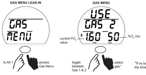
\*If no button is pressed the i100 will revert to the Dive Main screen after 10 seconds.
