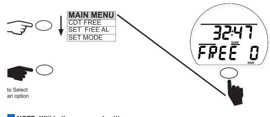
NOTE: Within the menu and settings screens the i100 will revert to the Free Surface Main screen after 30 seconds of inactivity.
