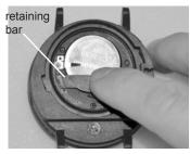
Battery Cover and Retaining Ring Installation
