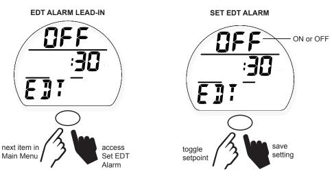
Factory set for a fixed 30 seconds, the EDT alarm sounds the audible alarm every 30 seconds
